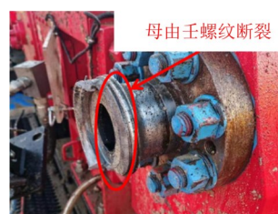
(a) 母由壬螺纹断裂
